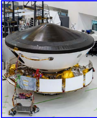
Mars 2020 heatshield and backshell (4.5 m)
